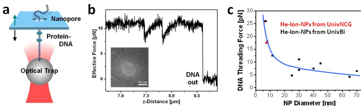
**Fig. 1. a)** Single molecule NP force spectroscopy: a microbead with an attached DNA molecule is optically trapped in the vicinity of a solid-state NP. A membrane voltage drives the negatively charged DNA into the NP. The
