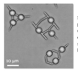
Some examples of nanotools used as AFM probes. Two-photon polymerisation has bee used to generate a range of structures, the designs of which were informed by detailed simulations of the EM field and hydrodynamics.
