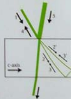
Figure 2: The signal beam 1 undergoes refraction and beam fanning. The phase-conjugated beam 4 is created by the fanned beams 2 and 3 (2' and 3') which are brought to overlap by total internal reflection at the crystal corner. The pump beam 5 transfers its energy to 1 by photorefractive two beam coupling.
